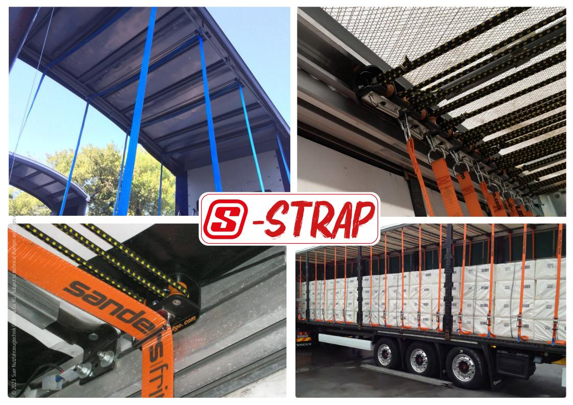
The S-Strap system enables fast, secure, and easy fastening and removal of loads on trucks with sliding tarpaulins. It is compatible with 50 mm wide DIN EN 12195-2 lashing straps.
