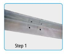
Drill two 6.2 mm holes for securing the aluminum piece. For M6 bolts, drill two 5 mm holes and tap the threads with an M6 tap into the profile.
