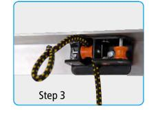
Pass the loop of the elastic through the hole in the center of the aluminum piece and pull it through the wheel along the bottom of the wheel to secure the elastic.
